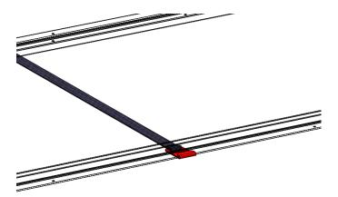
**Step 7:** Once the clips are attached to the panels pull the straps snug. Ensure that the field perimeter is square.
